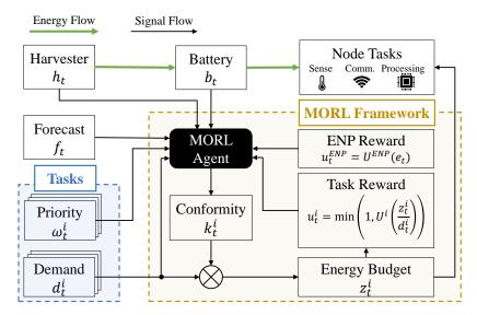
Figure 2. A general system model for multi-task EHWSNs.
