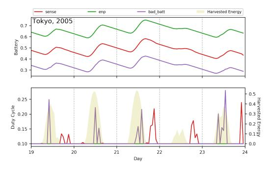
**Figure 9.** *bad\_batt* learns to accommodate for battery inefficiencies by maximizing duty cycles during the day. *sense* maximizes its duty cycle during the night depending on how much energy it was able to harvest during the day.
