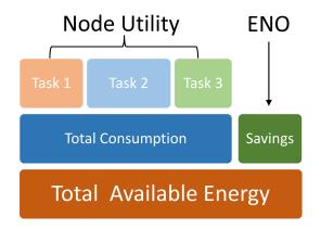
**Figure 1.** A multi-task EHWSN has to wisely determine its gross energy consumption at each time step so as to remain energy-neutral. Furthermore, it has to proportion the energy among different tasks to maximize node utility.
