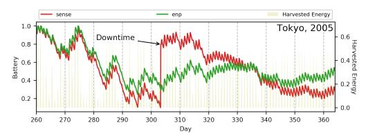
**Figure 8.** Battery traces for *sense*, *enp. sense* is more aggressive than *enp* when maximizing the sense-utility and therefore experiences downtime during winter. The sharp rise in battery level after a downtime signifies a node reset.
