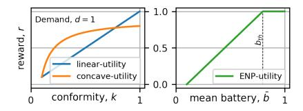
**Figure 5.** Linear and concave reward functions quantify the utilities for different tasks such as sensing, communication, and processing. The ENP-utility function indicates the long-term energy neutrality of the node.
