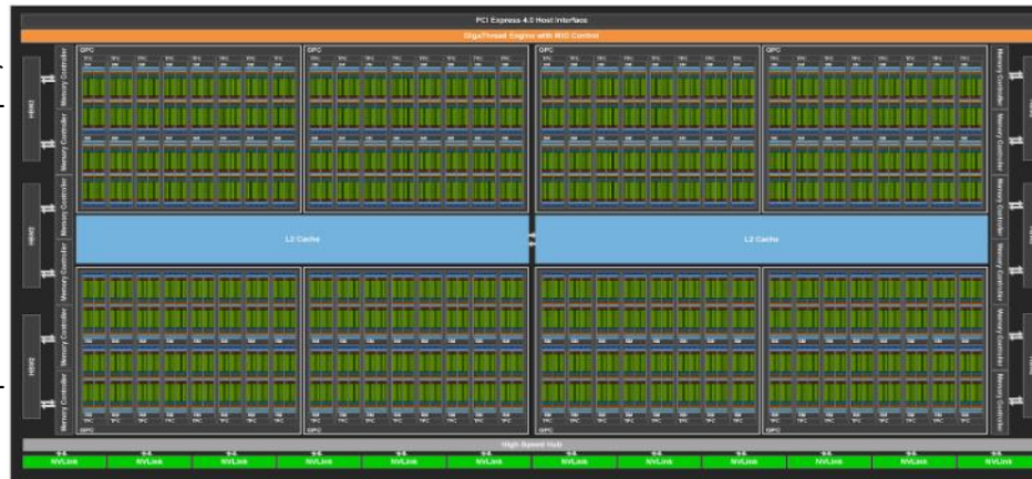
NVIDIA GA100 with 128 SMs. Each SM has multiple CUDA cores with INT32, FP32 and FP64 capabilities
